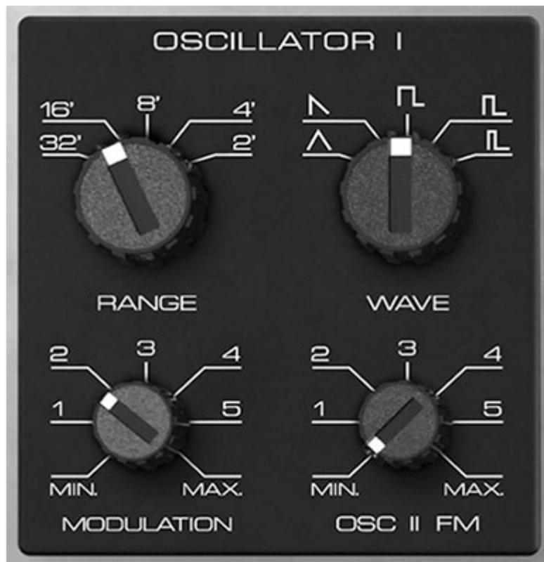
**Range**- Coarsely sets the signal generator pitch range in octaves. These are at standard organ footage settings of 32', 16', 8', 4', and 2'.
