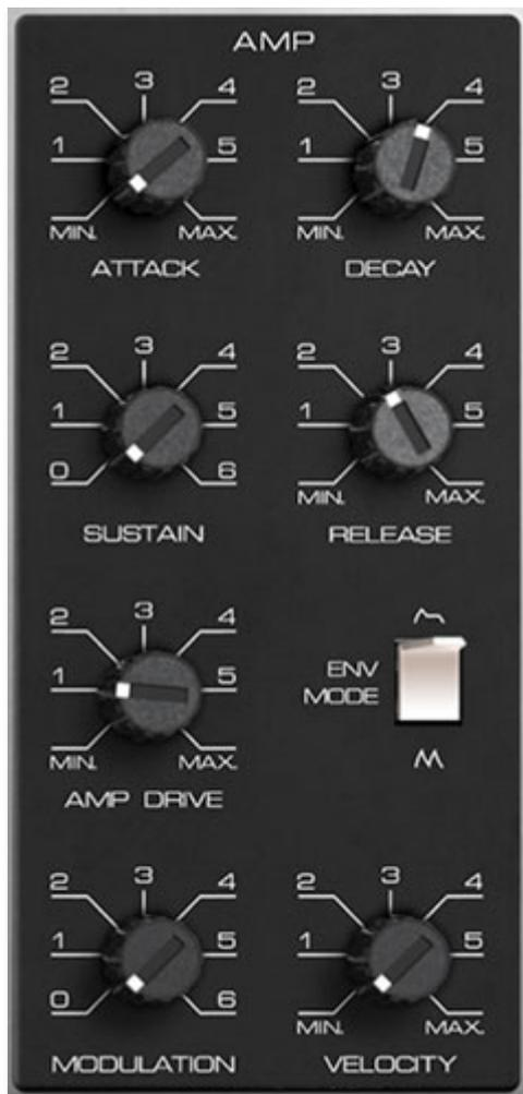
The Amp section controls overall amplitude (volume); this is mainly configured using the ADSR envelope generator, but controls for modulation amount and note velocity are also found here. .
