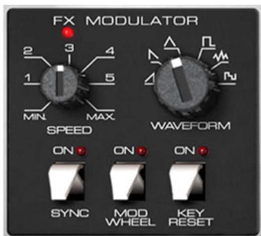
The FX Modulator section is a low-frequency oscillator that generates sub-audio range signals specifically for modulating effects parameters. **Though it appears in the same location and has similar controls, it operates completely independently of the Main page Modulator section.**
