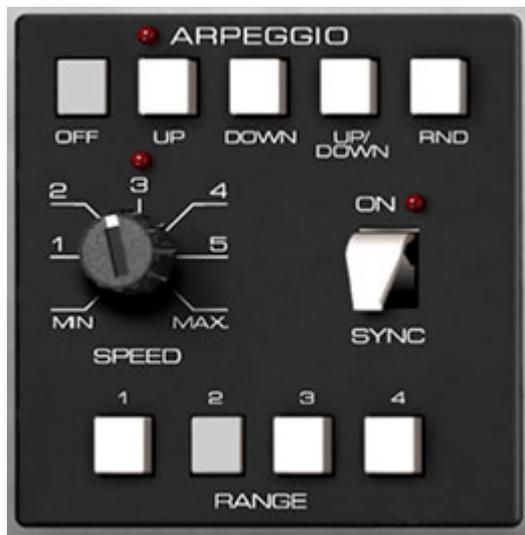
An arpeggiator is basically a step sequencer that plays each note of a chord individually in an ascending or descending pattern across one or more octaves.
