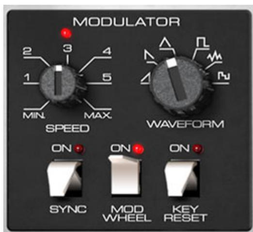
The Modulator section is a low-frequency oscillator that generates sub-audio range signals intended for modulation purposes. We've expanded on the original instrument in a couple of useful ways, including multiple modulation waveforms and tempo sync.
