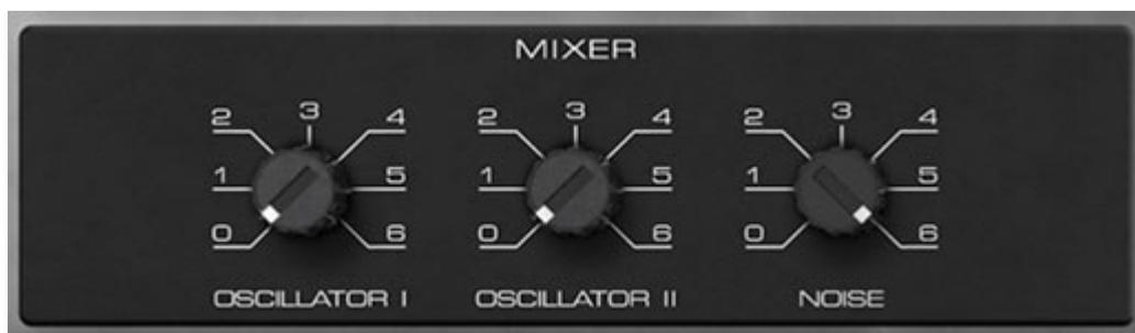
The Mixer section combines signals prior to the filter section.
