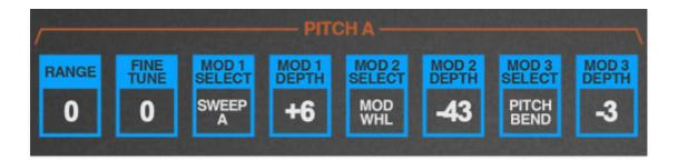
Each voice path includes a single oscillator; initial tuning and modulation are set in the PITCH section.
