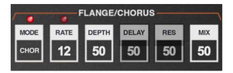
A thick and warm flange/chorus effect. Flanging and Chorus are closely related - the general difference being that flangers use a shorter time range and some amount of feedback (this intensifies the "jet-flyby" whoosh), whereas choruses utilize a slightly longer delay time, and no feedback.
