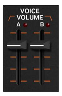
**VOICE VOLUME**- These sliders independently set the volume of each voice path. If the Single Layer Patch Config is currently selected, the *B* or *D* slider will be disabled and dimmed. Each of these has a red signal-present LED at the top; these very useful for determining which voice path(s) is currently making sound.
