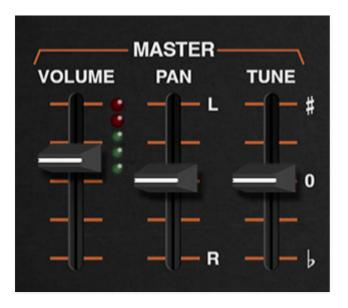
**VOLUME**- Sets the master volume for the entire instrument. The LED meter indicates output level; keep it in the high greens/low red to avoid undesirable digital clipping.
