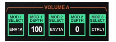
The VOLUME section defines how envelopes generators and other level modulation is applied to shape the amplitude of sounds using a voltagecontrolled amplifier (VCA). If you're not familiar with them, think of a VCA as a simple volume knob that gets automatically turned using control voltages.
