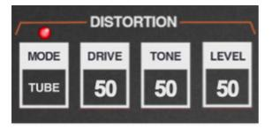
**MODE**- Turns distortion on and off and sets the type. The LED above the MODE button illuminates when distortion is enabled.
