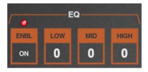
The EQ section precisely replicates the frequency and boost and cut characteristics of the original Chroma's three-band EQ - this is why some of the specs may look a little odd compared to more modern general-purpose EQ sections.
