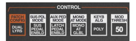
The CONTROL section contains what's often referred to as "global" parameters. Unlike all other PARAMETER PROGRAM controls, these apply to *both* voice paths - A/B for the Chroma or C/D for the Expander. This is why the word CONTROL (and most of the buttons) is white.
