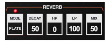
**MODE-** Turns the reverb effect on and off and sets the type. The LED above the MODE button illuminates when reverb is enabled.
