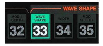
The teeny LED number display would show the current parameter number being adjusted and its value. In this case you'd choose value of 0, 1, 2, or 3 using the single *PARAMETER CONTROL* slider:
