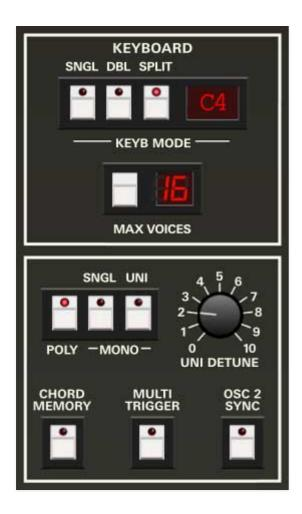
This section sets keyboard assignment and triggering behavior. This is divided into two sections - the upper frame controls are global, that is, they affect both the upper and lower layers. The bottom section parameters can be set independently for the upper and lower layers.
