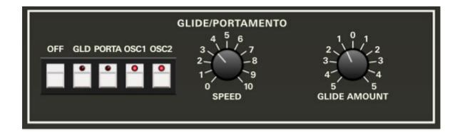
The original Elka instrument featured a unique implementation of note glide. "Glide" and "portamento" are often used interchangeably, but here "portamento" refers to the standard gradual pitch changes from note to note, whereas "glide" is what is more commonly referred to as a pitch envelope for each note played.
