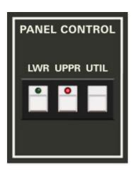
This innocuous little section is super important. As discussed in the **Keyboard** section, Elka-X can operate in three modes: *Single*, where one sound plays across the entire keyboard range, *Double*, where two separate sounds (layers) are stacked across the entire keyboard range, or *Split*, where two individual sounds are played above and below a user-specified split point (say that five times fast).
