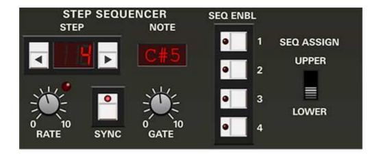
**Step buttons and display**- Each click of these buttons increments the current sequence step down or up respectively. Hold the mouse button down to move quickly through steps. We don't need yer dang carpal tunnel syndrome lawsuit, pal!
