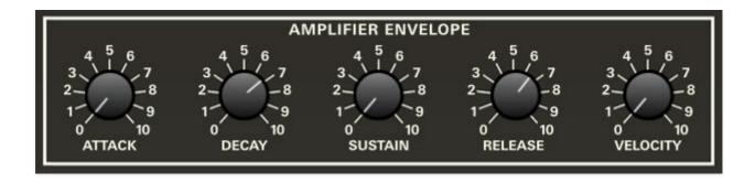
The Amplifier Envelope section consists of a standard attack, decay, sustain, release-style (ADSR) envelope generator controlling voltage-controlled amplifers (VCA's) for each voice.
