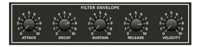
The Filter Envelope is a dedicated envelope generator for control of cutoff frequency (via the Envelope knob).
