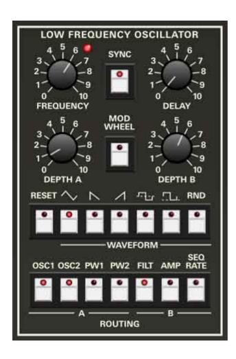
**Frequency**- The *Frequency* knob sets LFO speed , from 0.02 to 20 Hz (with *Sync* switch off). The LED beside the *Rate* knob flashes at the current modulation rate, and visually indicates the curve of the current mod waveform.
