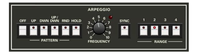
An arpeggiator is basically a step sequencer that plays each note of a chord individually in an ascending or descending pattern across one or more octaves.
