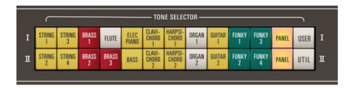
When in normal (factory preset) mode, clicking any of the buttons recalls the factory patch for the appropriate rank, and the Rank Voice Parameter controls instantly change to the correct positions.
