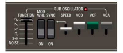
The Sub Oscillator generates sub-audio range signals intended for modulation purposes. It affects both currently active ranks (I/II or III/IV) equally.
