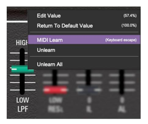
Begin by right-clicking on the green *LPF* slider in the Rank Voice Parameters *VCF* section and selecting *MIDI Learn.* A purple overlay appears over the slider indicating that it's in learn mode. Now move the desired hardware control device. The purple overlay disappears and the hardware control will move the onscreen slider. If you get cold feet (or accidentally put the wrong
