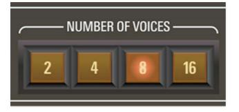
**2/4/8/16**- Sets the maximum number of notes that can simultaneously sound. Like the original instrument, there's no voice stealing. In other words, if the maximum number of voices are currently held down and new notes are struck, the new notes will *not* be audible until previously played keys are released.
