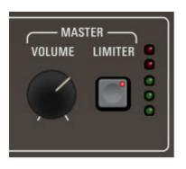
**Volume**- Controls the overall instrument volume.
