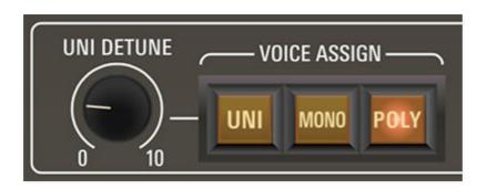
**Uni (Unison) Detune knob**- The *Uni Detune* knob is used in conjunction with the *Uni* Voice Assign mode to spread the tuning of the oscillators for fat sounds.
