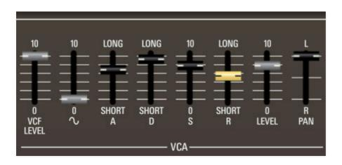
VCA stands for "voltage-controlled amplifier. Here you'll set incoming and outgoing volume, as well as amplitude envelope parameters.
