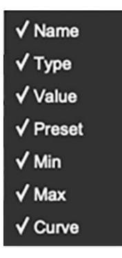
Right-clicking anywhere in the top row (*Name, Type, Value*, etc.) displays the column configuration menu. Checking/unchecking these allows hiding and display of each column. This has no effect on assignments.
