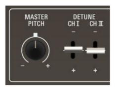
**Master Pitch-** Sets pitch globally for the entire instrument up or down a half-step.
