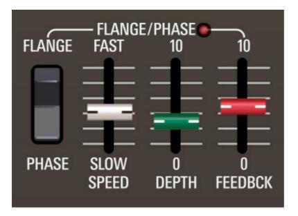
The familiar "jet-plane" flange or super swooshy phase modulation effects. Both effects are mono, but layer panning positions are properly maintained.
