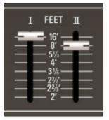
**Feet I/II/III/IV**- Sets the coarse pitch range for each oscillator in traditional organ footage settings of *16'*, *8'*, *5 1/3'*, *4'*, *3 1/5'*, *2 2/7'*, *2 2/3'* and *2'*. The 3 *1/5'* and 2 2/7' footages are from GX-1; these are not available on the original CS-80.
