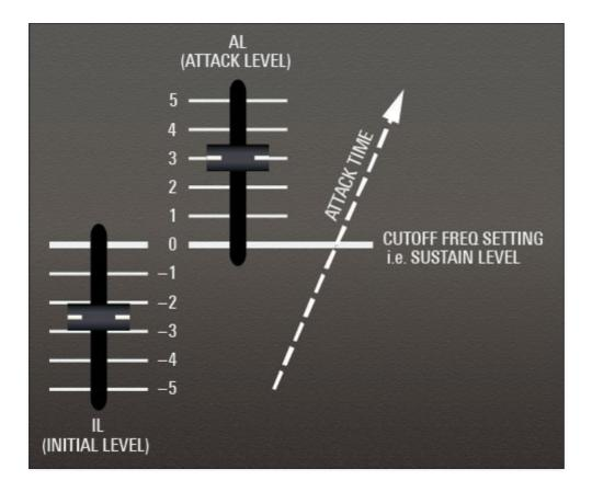
To achieve a typical attack/release envelope shape, where the envelope rises to the sustain level and then falls back when the key is released, raise the *IL* slider (more negative) and leave *AL* at zero. To get an attack/decay function, where the envelope rises and then falls back while the key is still down, raise the *AL* slider (more positive) and leave *IL* at zero. Other combinations of *IL* and AL settings will result in ADSR functions of different sizes.
