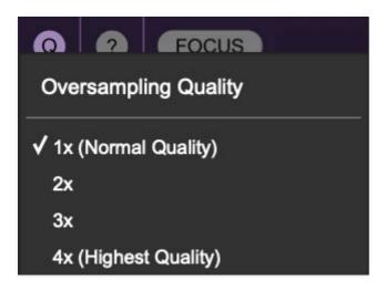
**Q Oversampling Quality -** The Q button sets GX-80's internal oversampling rate; the higher the setting, the better audio fidelity will be, with the caveat that more computer processing power will be required.
