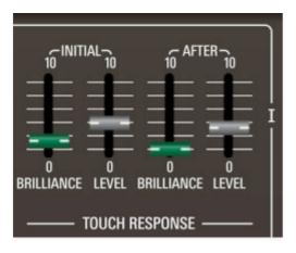
The Touch Response section allows polyphonic control of lowpass and highpass cutoff frequencies as well as amplitude via keyboard velocity and aftertouch.
