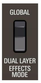
**Effects Mode**- When set to the *Dual Layer* position, an entirely independent effects section is available for the upper and lower layers. When set to the *Global* position, both layers (i.e., voice ranks I/II/III/IV) run through a single set of effects. This is useful when creating patches that combine all four voice ranks into one overall sound, or when creating a split sound and you'd like the same effects settings for both layers.
