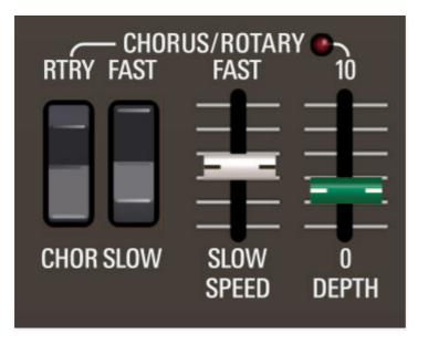
This can function as a rotary speaker effect or a chorus. Note that these are totally different effects - the rotary speaker is a true Leslie emulator, with all the inherent quirks of a real rotating speaker cab miked in stereo. Meanwhile, the chorus effect is not an emulation of the CS-80's onboard chorus, because frankly, the original chorus fidelity wasn't all that good, so we've improved it considerably. Both the chorus and rotary effects are full stereo.
