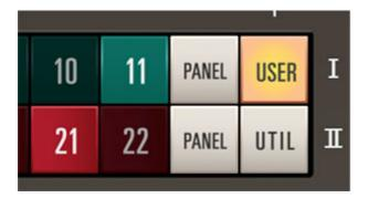
**User bank button**- The *User* presets allow saving or recall of the voice parameters *for that rank only*. This is useful for quickly creating and experimenting with composite sounds from multiple ranks. The 11 presets per bank (22 total) are intended for user favorites and will remain in GX-80's
