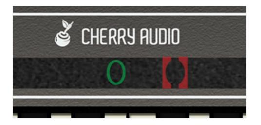
To use the ribbon, click and hold the mouse button or trackpad and move right or left. The green oval indicates the "home" nominal pitch position, and the red brackets will move left or right as the mouse is moved. The brackets turn green when aligned over the oval, indicating that pitch is "home." If the button is released at any time, pitch will instantly snap back to normal.
