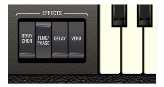
On/off status is set for each effect using the rocker switches immediately to the left of the keyboard. Like other GX controls, the down position corresponds to on. LEDs next to each effect name also indicate on/off status.
