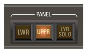
Because displaying the controls for four sets of Rank Voice Parameters would have made the UI enormous, GX-80's panel displays two sets of Rank Voice Parameters like a CS-80. These are referred to as Upper (voice ranks / and //) and Lower (voice ranks /// and //).
