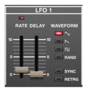
LFO 1 (low-frequency oscillator ) generates sub-audio range signals intended for modulation purposes.
