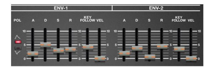
Like the original Jupiter-6, Mercury-6 includes two ADSR envelope generators. Envelope 2 is mostly dedicated to controlling note amplitude; Envelope 1 generally controls filter cutoff frequency, but both include few additional modulation routings. Before we get into their controls, let's review the operation of an ADSR envelope.
