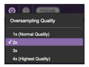
**Oversampling Quality (Q)-** The Q button sets Mercury 6's internal oversampling rate; the higher the setting, the better audio fidelity will be, with the caveat that more computer processing power will be required.
