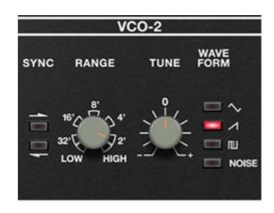
**Range**- Sets the basic pitch range of the oscillator from *Low* (below audible range), through 32' to 2' footages, up to *High* (above audio range). The knob moves continuously, but discretely snaps to each range. The *Low* and *High* settings are intended for use with the Cross Mod functions described above (i.e., using VCO-2 as a mod source). When using VCO-2 for mod, we recommend disabling its audio output by dialing the adjacent Mixer knob all the way to *VCO-1*.
