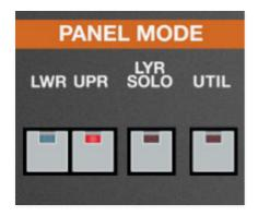
This innocuous little section is super important. As explained above, Mercury-6 can operate in three modes: *Whole,* where one sound plays across the entire keyboard range, *Layer*, where two separate sounds (layers) are stacked across the entire keyboard range, or *Split*, where two individual sounds are played above and below a user-specified split point.
