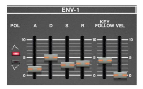
Envelope 1 is mainly intended to control filter cutoff frequency, but it also can be routed to control oscillator pulse-width modulation.
