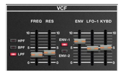
The VCF section consists of a multimode filter with a 24 dB/oct lowpass, 24 dB/oct highpass, or 12 dB/oct bandpass modes.
