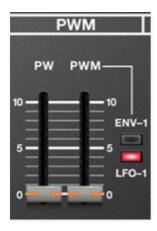
These controls determine the pulse wave width or "duty-cycle" when the pulse wave is selected (shown above) on one or both oscillators.
