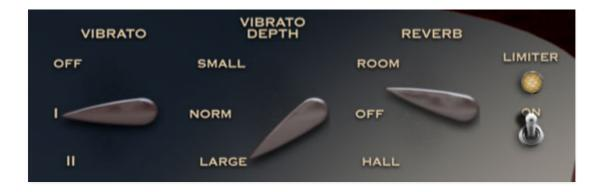
**Vibrato**- Enables the Novachord's unique vibrato circuit. *Vibrato I* uses square-wave modulation, as used in the earliest Novachord models; *Vibrato II* makes use of a more rounded-off square wave, as used in later Novachords.
