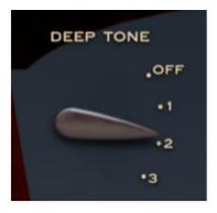
**Deep Tone**- Sets the level of tone generator signal with a one-pole (6dB peroctave slope) lowpass filter with a fixed frequency of 160 Hz applied.
