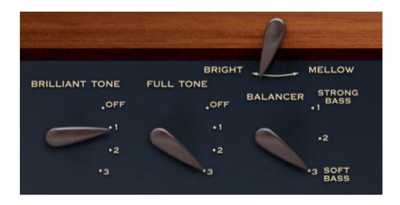
**Brilliant Tone**- Sets the level of tone generator signal with a one-pole (6dB per-octave slope) highpass filter with a fixed frequency of 2000 Hz applied.
