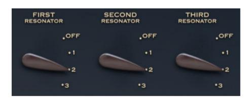
The three resonators are bandpass filters, operating consecutively in low, mid, high frequency ranges.
