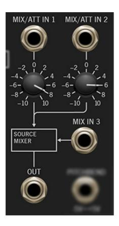
We've added a three-input mixer/attenuator/inverter that's really handy. It can be used for mixing audio or control signals, or as a simple attenuator if a single signal is routed through it.
