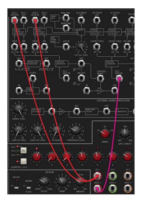
The patch shown above is good starting point. It uses the first sequencer channel with  $CV\ 1$  patched to VCO 1 and VCO 2  $Keyb\ In$  jacks to control pitch, and the  $Gate\ 1$  jack patched to the  $EG\ 2$   $Gate\ In$  jack. Once you have it patched, click the Start/Stop button, and turn the knobs to hear varying pitches. You may want to experiment with pitch range and octaves using the VCO Scale knobs and sequencer Range knob, respectively.
