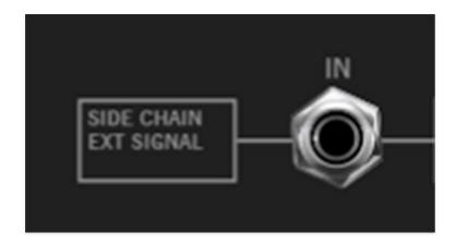
Once you've successfully routed the sidechain input signal, it will be normalled into the *External Signal Processor* (hence the little box that says *Side Chain Ext Signal* at the left).
