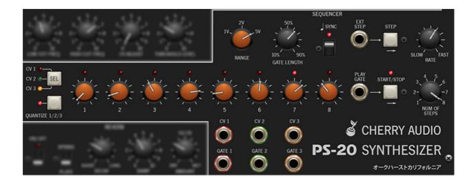
PS-20 features a three-channel, eight-step sequencer - it actually is three completely independent eight-step sequencers, each with its own pitch and gate outputs. Each channel is color coded to make using it a snap.
