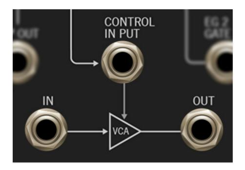
The patch panel section also includes a "bonus" auxiliary VCA. Its main purpose on the original MS-20 was to allow modulation generator amount to be controlled via EG 1 or with a mod wheel. But with PS-20's additional patch panel I/O, it's possible to use the auxiliary VCA to create complex, "dual voice" patches, typically in conjunction with one more sequencer layers.
