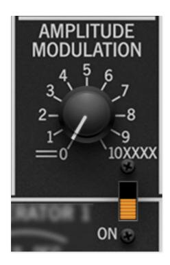
**Amplitude Modulation knob and routing switch**- Moving a little further down the panel, Amplitude Modulation allows Mod Generator 1 to modulate audio level (make sure the orange switch between the sections is in the down position). At slower mod speeds, this is useful for conventional undulating-level tremolo effects. When the Mod Generator 1 is set to faster speeds, you'll hear ring modulator-type special effects (try experimenting with different Mod Generator waveforms as well).
