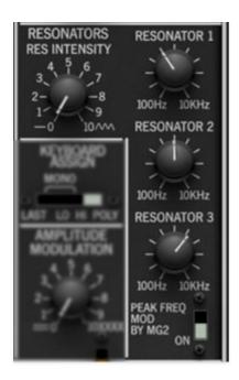
The Resonators section is set of three 12 dB/oct bandpass filters with a high amount of resonance (hence the clever name). The use of "vactrols" (aka, light-controlled resistors) in the original instrument gave these a pleasantly gooey, phaser-like tone. We've reproduced it super-accurately, if we say so ourselves.
