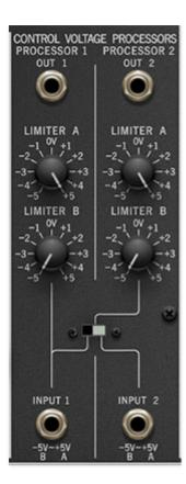
Like the many analog synthesizers, PS-3300 makes use of control voltages ranging from -5V  $\sim$  +5V. These voltages are used to control oscillator pitch and vibrato, filter cutoff, amp modulation and more. The Control Voltage Processors primary purpose is to control voltage ranges or "swing." (not the kind of swing heard in Bobby Brown songs in the late 80s).
