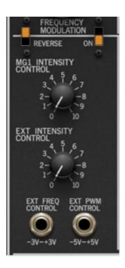
**Reverse switch-** Enabling the *Reverse* slide switch inverts the polarity of both the hardwired *Mod Generator 1 and Ext Freq Control* signals.
