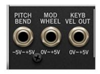
**Pitch Bend**- This outputs a voltage between -5V  $\sim$  +5V when the pitch wheel or joystick on a MIDI/USB controller is moved. Its output nominally sits at 0V.
