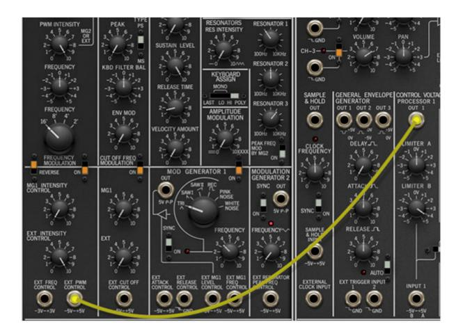
The MG2>PWM routing can be overridden to create a constant, non-modulated pulse width by using one of the Control Voltage Processors in the Master Panel. Route a cable from the Control Voltage Processor Out 1 or Out 2 jack to the Ext PWM Control jack at the bottom of the Signal Generators section. Set PWM Intensity and Ext Intensity Control knobs to max. The CV Processors Limiter B knob can now be used to vary pulse-width.
