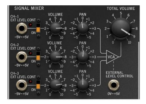
The Signal Mixer is where volume and panning is set for the three Voice Panels "channels."
