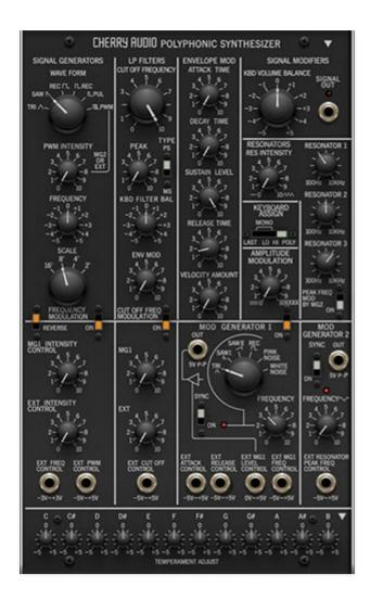
The PS-3300 includes three identical polyphonic Voice Panels. Each of the three Voice Panels is essentially an independent single-oscillator polyphonic synth. Each one consists of a signal generator (Korg's silly name for an oscillator), a lowpass filter, an ADSR envelope generator, two Mod Generators (Korg's also-silly name for an LFO), and a "Resonators" section. In the following pages, we'll go over all Voice Panel parameters.
