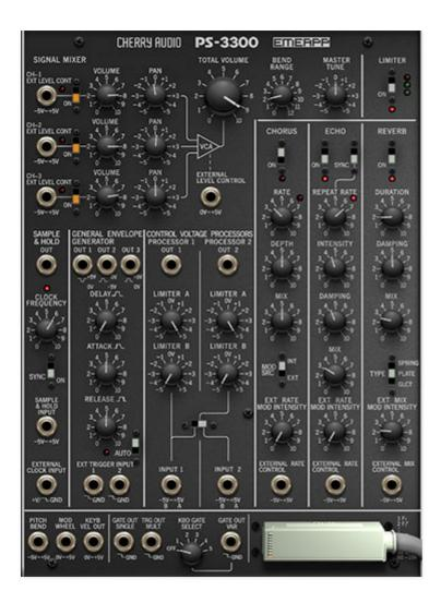
The Master Panel includes a mixer, additional "mono" processing modules (sample & hold, an additional utility envelope generator, CV processors, and
