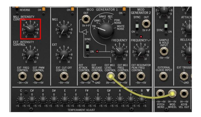
**Ext MG1 Freq Control jack**- Allows a CV to control Mod Generator 1's frequency. This is a bipolar input that accepts CV's from -5V to +5V; negative CV's will decrease mod rate and positive CV's will increase mod rate.
