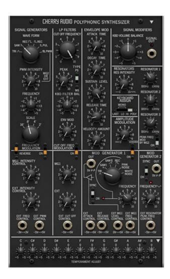
Each of the three Voice Panels can be thought of as a totally independent single-oscillator polyphonic synth. Each one consists of a signal generator (Korg's silly name for an oscillator), a lowpass filter, an ADSR envelope generator, two Mod Generators (Korg's also-silly name for an LFO), and a "Resonators" section. We'll discuss it more later on, but the PS-3300's Resonators section is really unique, and amongst other things, it makes super fabulous phaser-type sounds.
