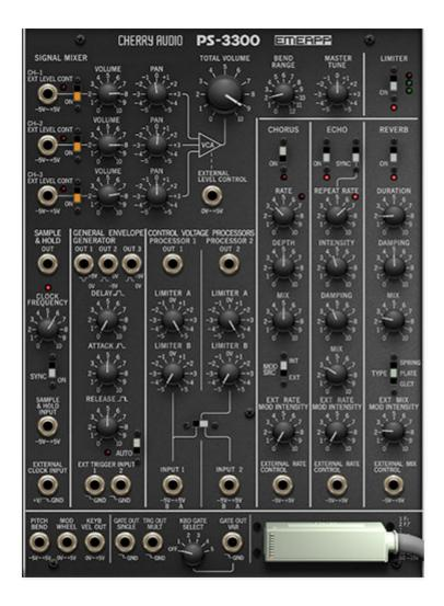
The Master Panel on the right side includes a mixer for all three Voice Panels, the Sample & Hold generator, the General Envelope Generator, two Control Voltage Processors, keyboard-related CV outs and controls, and audio effects including Chorus, Echo, Reverb, a Master Limiter, and master controls for volume, tuning, and bend range. Oh yes, and an enormous plug that doesn't do anything, but it looks super cool.
