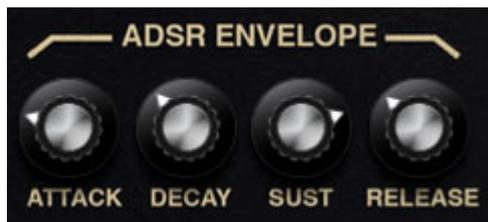
**Attack**- Defines the length of time for voltage to rise from 0V to 5V when a key is played.
