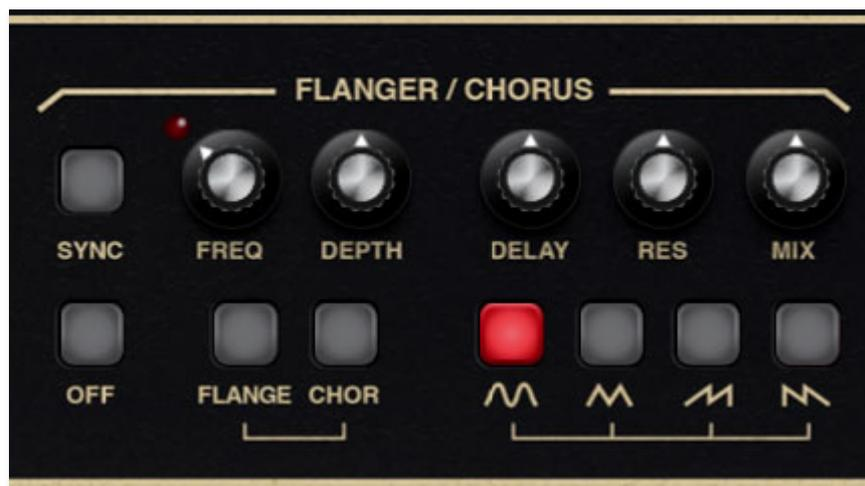
We've included a thick and warm flanger/chorus effect. Flanging and Chorus are closely related - the general difference being that flangers use a shorter time range and some amount of feedback (this intensifies the "jet-flyby" whoosh), whereas choruses utilize a slightly longer delay time, and no feedback.
