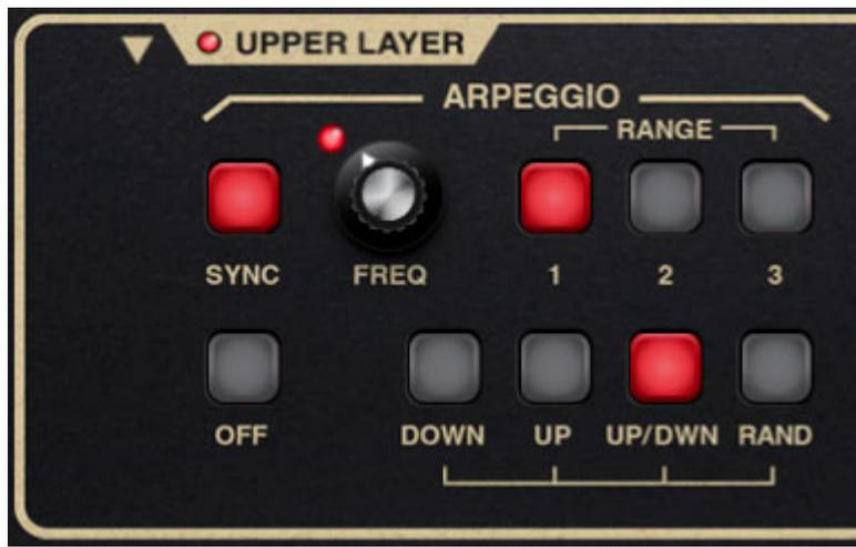
An arpeggiator is basically a step sequencer that plays each note of a chord individually in an ascending or descending pattern across one or more octaves.
