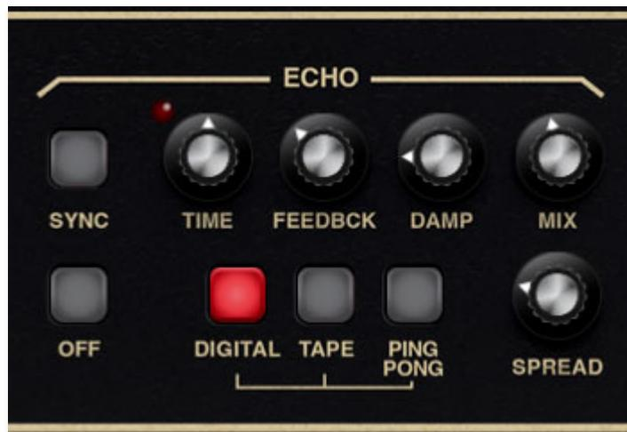
**Sync**- The *Sync* button locks the delay time to master tempo. When engaged, the *Time* knob snaps to note values ranging from 1/64th note triplet to 8 beats. *Sync* mode locks to the tempo in the top toolbar when using the Pro Soloist standalone version or the current project tempo when the plug-in version is used in a DAW.
