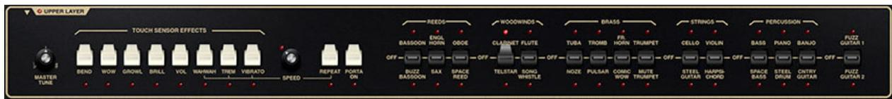
This is the the primary panel mode, intentionally designed to closely emulate the original Pro Soloist panel control configuration. Here you'll select from the Pro Soloist "factory" paddle-switch presets, and enable the Touch Sensor aftertouch controls, "wahwah" and vibrato mod, and more.
