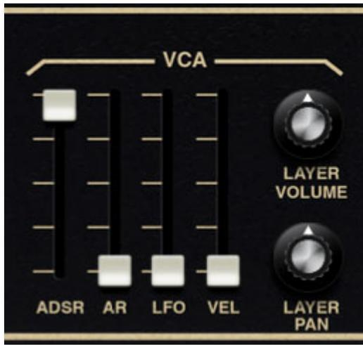
VCA is short for “voltage-controlled amplifier,” and for all intents and purposes, you can think of it as the automated volume knob that controls the amplitude of each note played. It has a number of mod sources, but is primarily controlled by either the ADSR or AR envelope generator.
