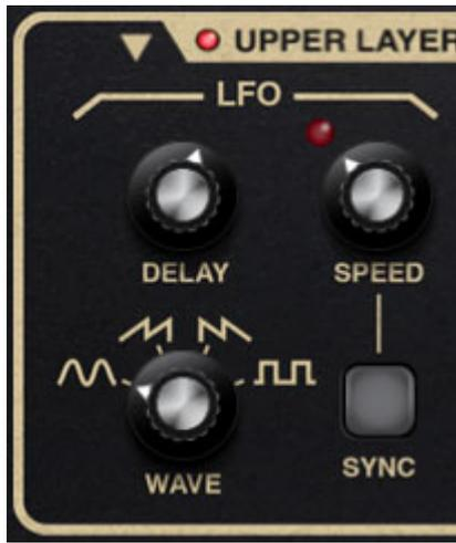
The LFO (low-frequency oscillator ) generates sub-audio range signals intended for modulation purposes.
