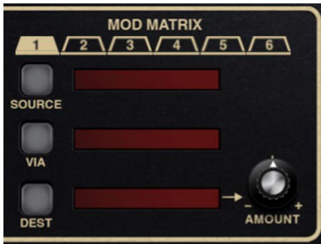
Pro Soloist's modulation routings are extensive and super easy to use. Each of its six mod slots have source, via, and destination popup menus and a bipolar attenuator to adjust the amount of mod.
