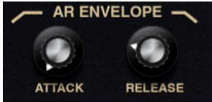
**Attack**- Defines the length of time for voltage to rise from 0V to 5V when the gate voltage is applied.
