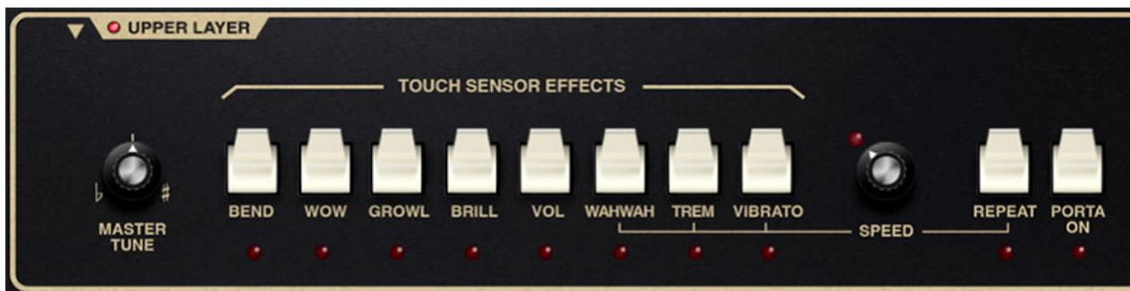
**Bend**- Enables upward pitch bend via aftertouch.
