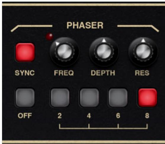
**Sync**- The *Sync* button locks the rate of the Phaser's modulation LFO to the tempo in the top toolbar when using the Pro Soloist standalone version, or to the current project tempo when the plug-in version is used in a DAW. When engaged, the *Freq* knob snaps to note values ranging from 1/64th note triplet to 8 beats.
