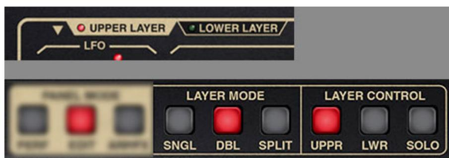
These tabs and buttons select which layer's Panel Controls are currently viewed and editable when *Double* or *Split* Layer Mode is enabled. If *Single* mode is currently selected, only the Upper layer plays, and the Layer Control buttons aren't needed. When *Single* mode is selected, the Layer Control
