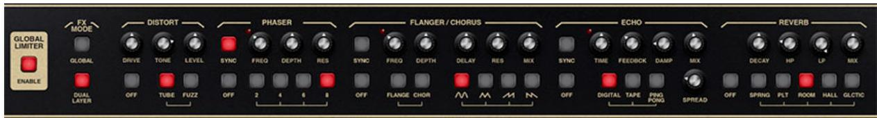
Pro Soloist includes six simultaneous effects: Distortion, Phaser, Flanger/Chorus, Delay, and Reverb. These can be used in any combination.
