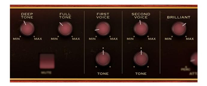
The *Deep Tone*, *Full Tone*, *First Voice*, *Second Voice*, and *Brilliant* knobs each control various filtered versions of the basic Solovox oscillator tone. Unlike typical analog synthesizer filters, the oscillator signal is split and routed to *all* of the filters, processed and then summed together, creating a composite tone, so it's best to think of these knobs as mixer controls. If all of the Tone knobs are set to zero, no sound is heard.
