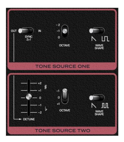
As monophonic analog synths go, MG-1 Plus is unique in that if features two standard mono analog oscillators (i.e., capable of sounding one note at a time), as well as a poly section that can sound up to 32 notes simultaneously. In this section, we'll discuss the mono oscillators. Note that the MG-1 front panel refers to oscillators as "tone sources;" perhaps Radio Shack felt this would be less intimidating for consumers than, "oscillator."
