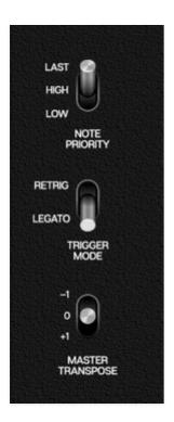
**Note Priority**- Since the Tone Generators are monophonic (i.e. they can only play one note at a time), this control determines which note will sound if more then one key is played simultaneously.
