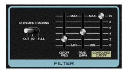
The Filter section is a 24 db/oct lowpass filter that removes high frequencies as its cutoff frequency setting is decreased from max, resulting in a dulling of sound. This a version of the classic transistor "ladder" filter, renowned for its meaty, fat sound.
