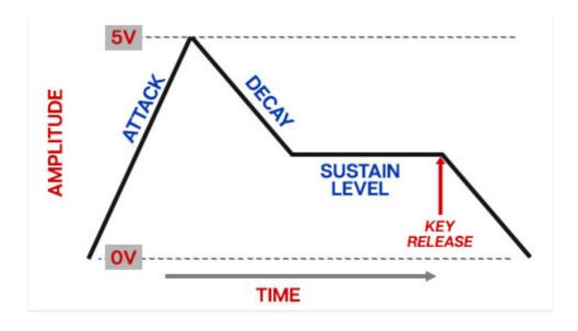
When a voice sees a gate voltage from a note, the envelope outputs a dynamically changing voltage, according to the settings of its stages.
