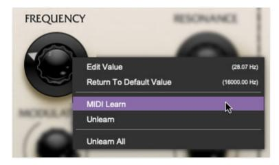
Begin by right-clicking on the *Fc* slider in the *VCF* section and selecting *MIDI Learn.* A transparent purple overlay appears over the knob indicating that it's in learn mode. Now move the desired hardware control device. The purple overlay disappears and the hardware control will move the onscreen slider. If you get cold feet (or accidentally put the wrong control into learn mode), learn mode can be aborted by right-clicking and selecting *Stop Learning*.
