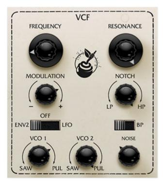
**Frequency**- Sets the frequency where frequency attenuation begins with its effect dependent upon the currently chosen lowpass/bandpass/notch/highpass/etc. filter mode.
