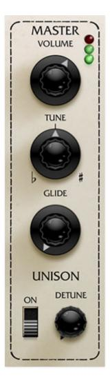
**Volume and meter**- Sets overall volume. The meter should be kept "in the green" to avoid ugly digital clipping.
