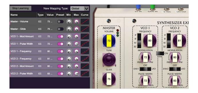
When in MIDI learn mode, any previously assigned controller numbers will show in squares. These indicate the MIDI continuous controller number of the assigned hardware control (these are also displayed in the *MIDI* library tab at left).
